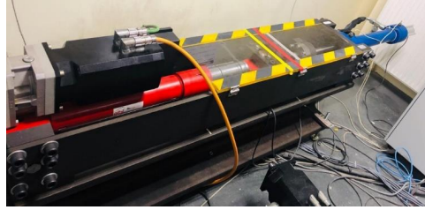
Figure 2: EHA-EMA test rig
