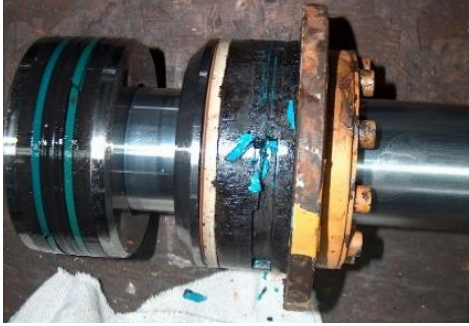
Figure 1: Sealing of the hydraulic cylinder, whose material became brittle due to high temperature
