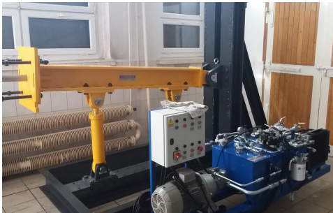
Figure 5: Test stand for testing hydraulic cylinders
