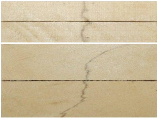
Figure 4: Zone line formed by a Lt/Th I dual culture in a maple sample.
