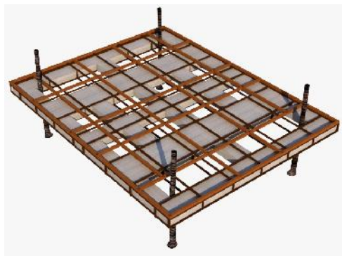
Figure 4. Placement detail of Styrofoam as the floating foundation material (as many as 56 sheets)
