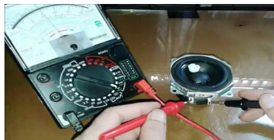
Gambar 8. Pengujian loud speaker
