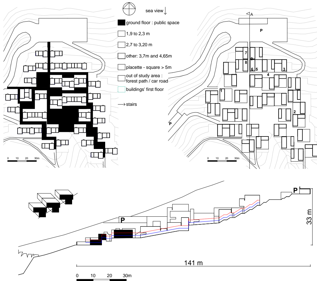
Figure 5. Merlier. Left: ground floor: partial underground units, public pedestrian space in black Right: first floor plan: pedestrian street widths and SVF locations Bottom left: schematic diagram of the grid assembly of units on a slope; Bottom right: Section A. Red line: mean building height; Blue line: Absolute Rugosity or mean urban canopy height
