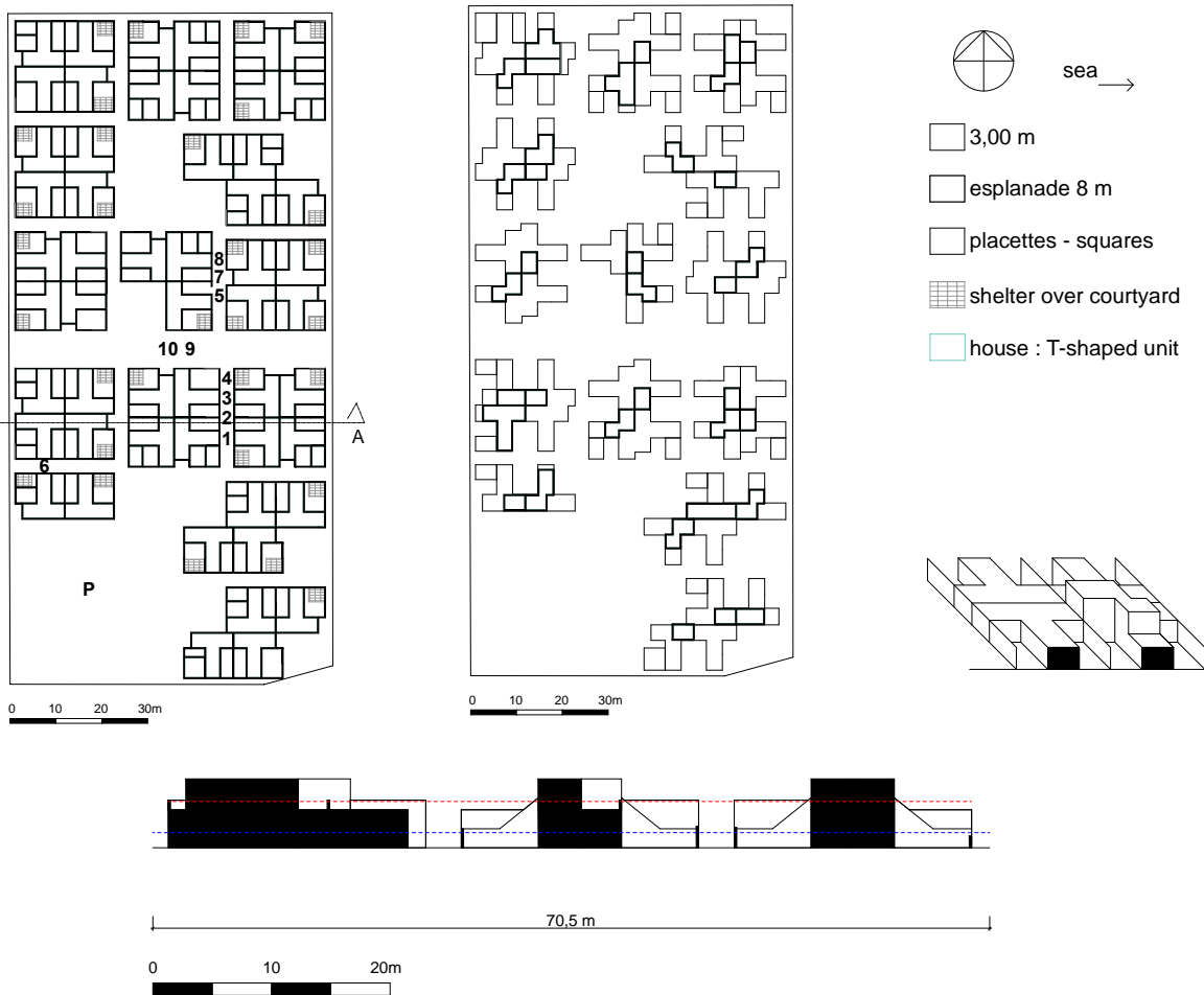
Figure 2. Village Grec. Left: Ground floor with pedestrian street widths and SVF locations; Middle: first floor Right: schematic diagram of the assembled "T" units Bottom: Section A. Red line: mean building height; Blue line: Absolute Rugosity or mean urban canopy height
