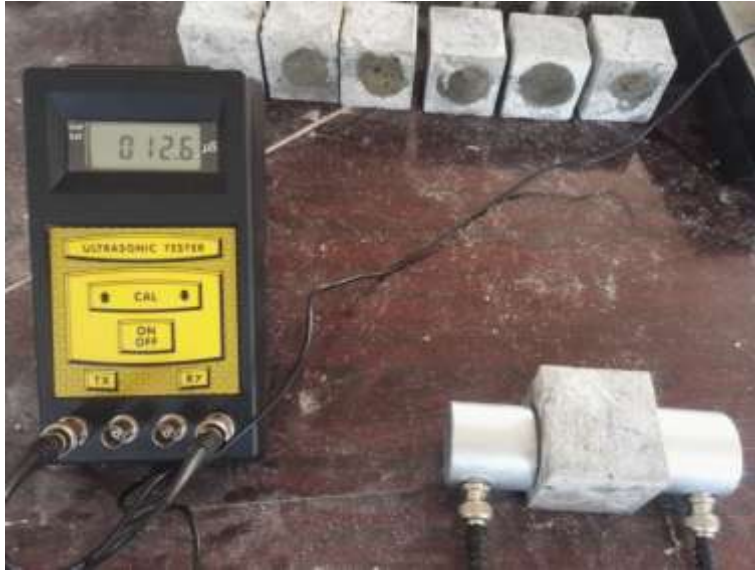
Figure 4: The ultrasonic pulse velocity test of mortar cubes.
