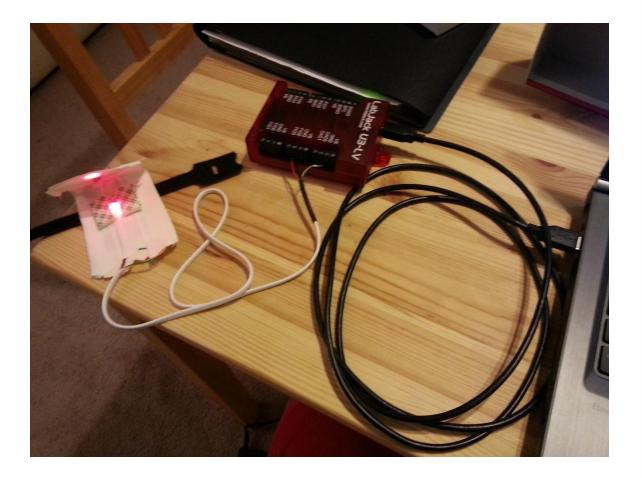
Heart rate apparatus with photoresist or and LED. Picture by National Instruments [4]. The complete system
