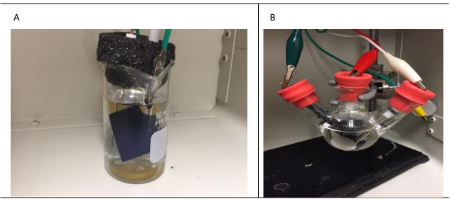
**Figure 7.** (A)Electrochemical setup and polymerization of Thiophene using CV from 1.6 to 1.8 V at a sweep rate of 0.01 V. (B) Three electrode cell consisting of gold working electrode, platinum wire counter electrode and Ag/AgCl reference electrode.
