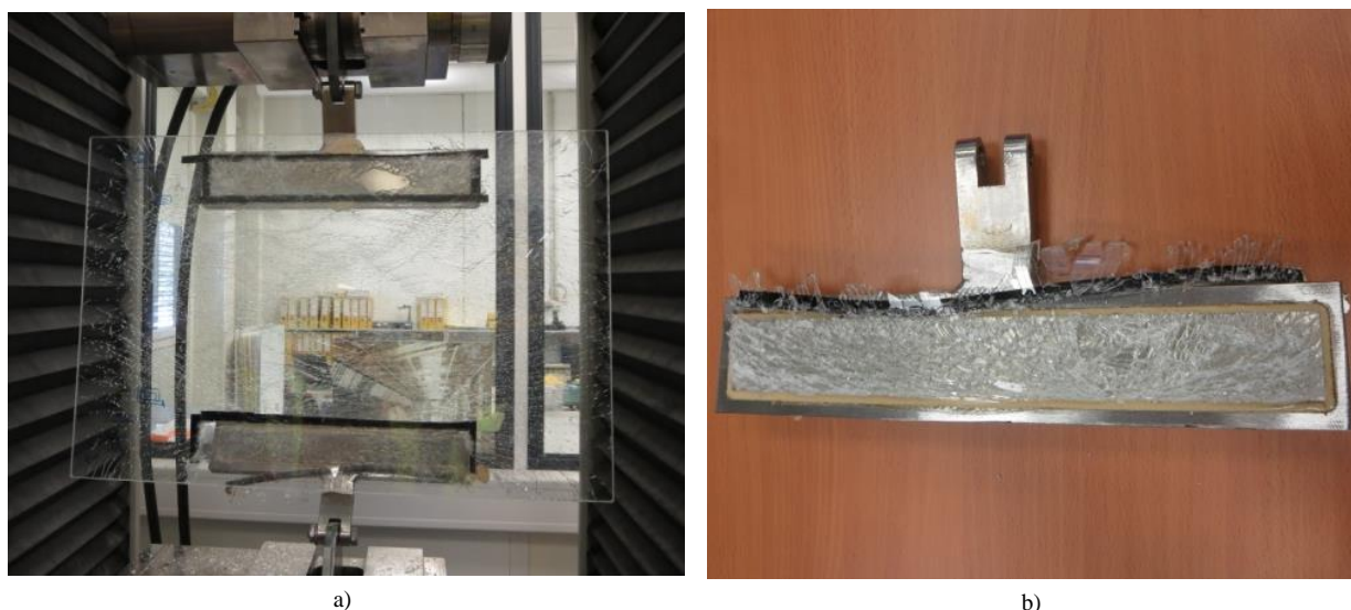
Fig. 15a) Glass sample after failure, b) Adhesive layer covered with glass fragments. (© seele).
