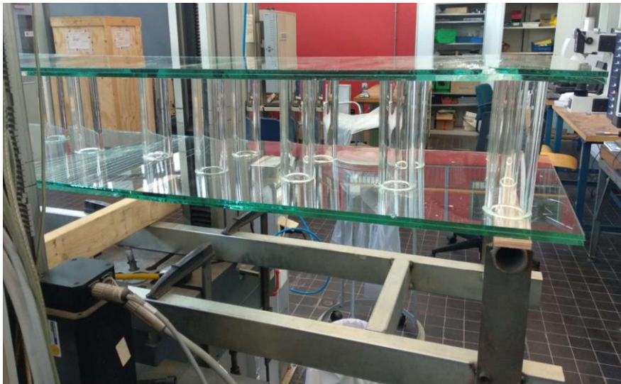
Fig. 8 Testing of prototype panel.
