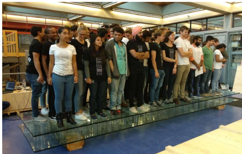
Fig. 14 Non-destructive test of large prototype panel using a static load exceeding the normal service load.
