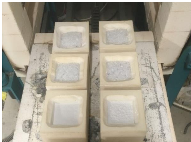
Fig. 5 Molds inside the oven ready for the firing.
