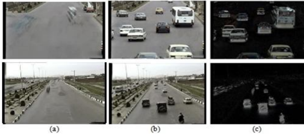
Fig. 2- (a) Generated Background image. (b) A sample frame of a video sequence. (c) Extracted foreground frame
