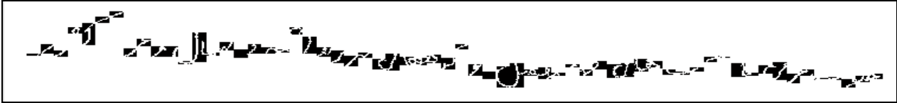
Fig.5. Text-line image after selecting black rectangles with maximum heights in each strip and mapping the original text-line image on the selected black areas and finding candidate points
