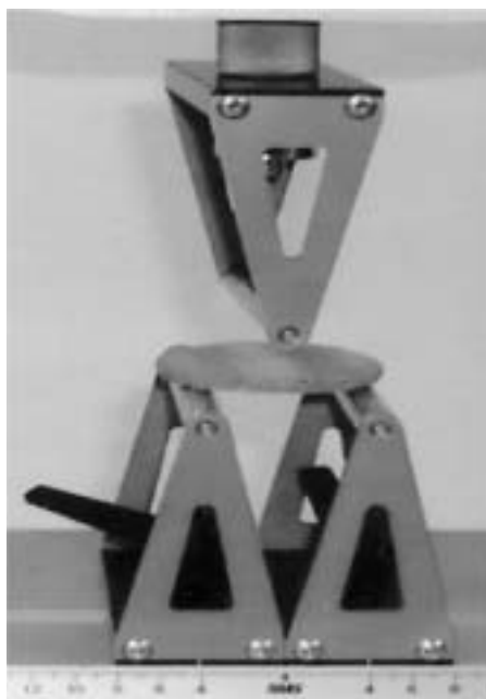
Figure 1 Photograph of placement of biscuit on the beam for the textural measurement.
