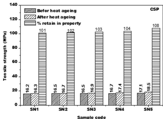
FIG. 3. Tensile strength of the NBR/SBR (50/50) blend and (NBR/SBR)/CSP/CN nanocomposites.
