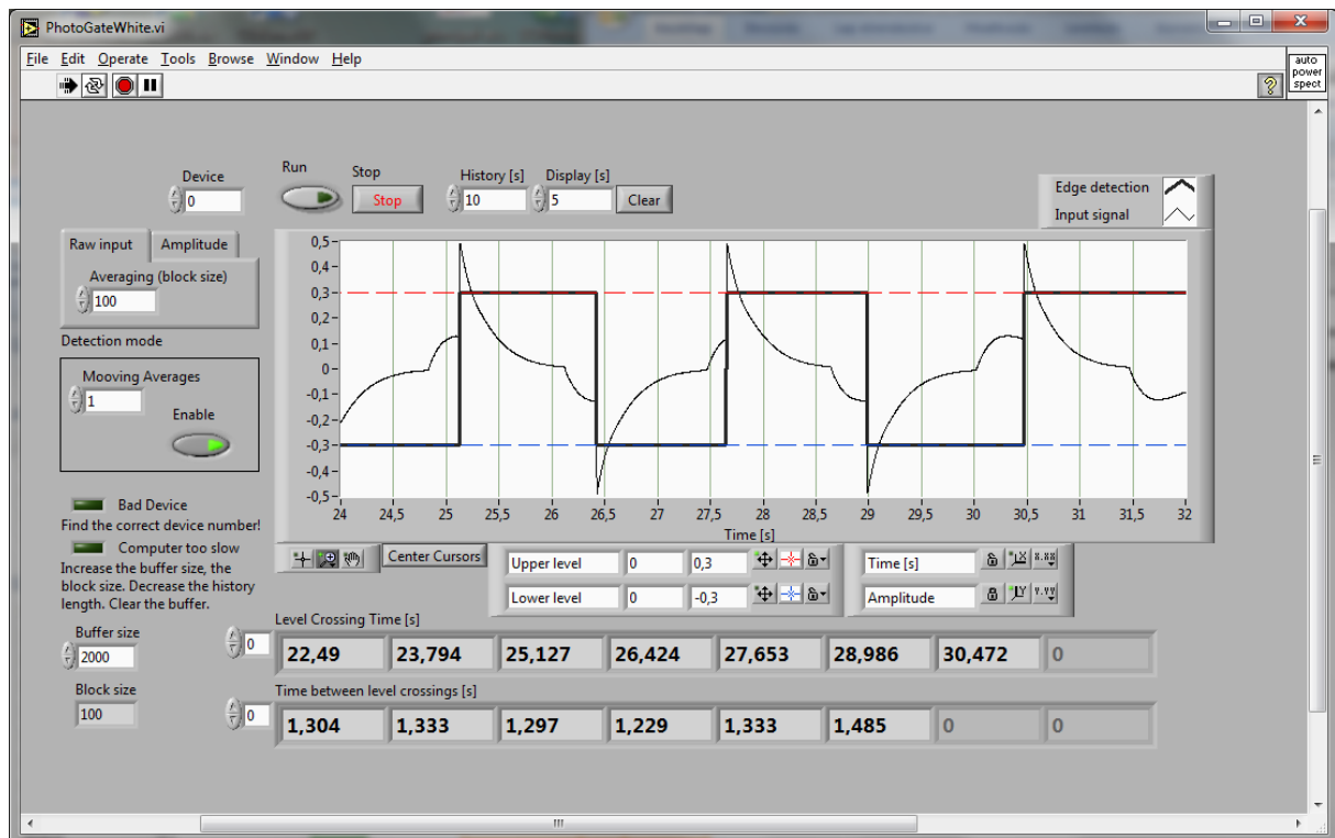
Figure 24. Photogate software developed in LabVIEW.
