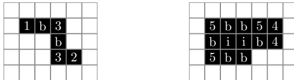
Figure 3: Examples of endpoints. Points marked “k” are endpoints of type Ei ( k = 1, \dots, 5; i = k, \dots, 5 ). Points marked “i” are interior points, while points marked “b” are border points that are not endpoints.
