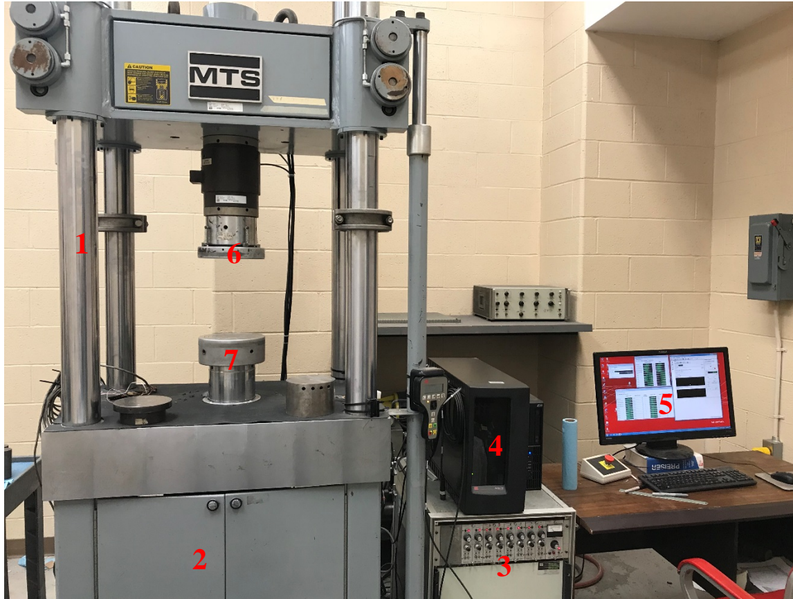
Figure 15. MTS servo-controlled compression testing system and its components- (1) Load frame (2) Hydraulic actuator (3) Strain gauge control panel (4) MTS data acquisition system (5) Computer (6) Upper steel platen (7) Lower steel platen
