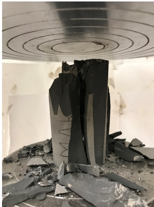
Figure 17. Axial splitting failure of shale observed post failure
