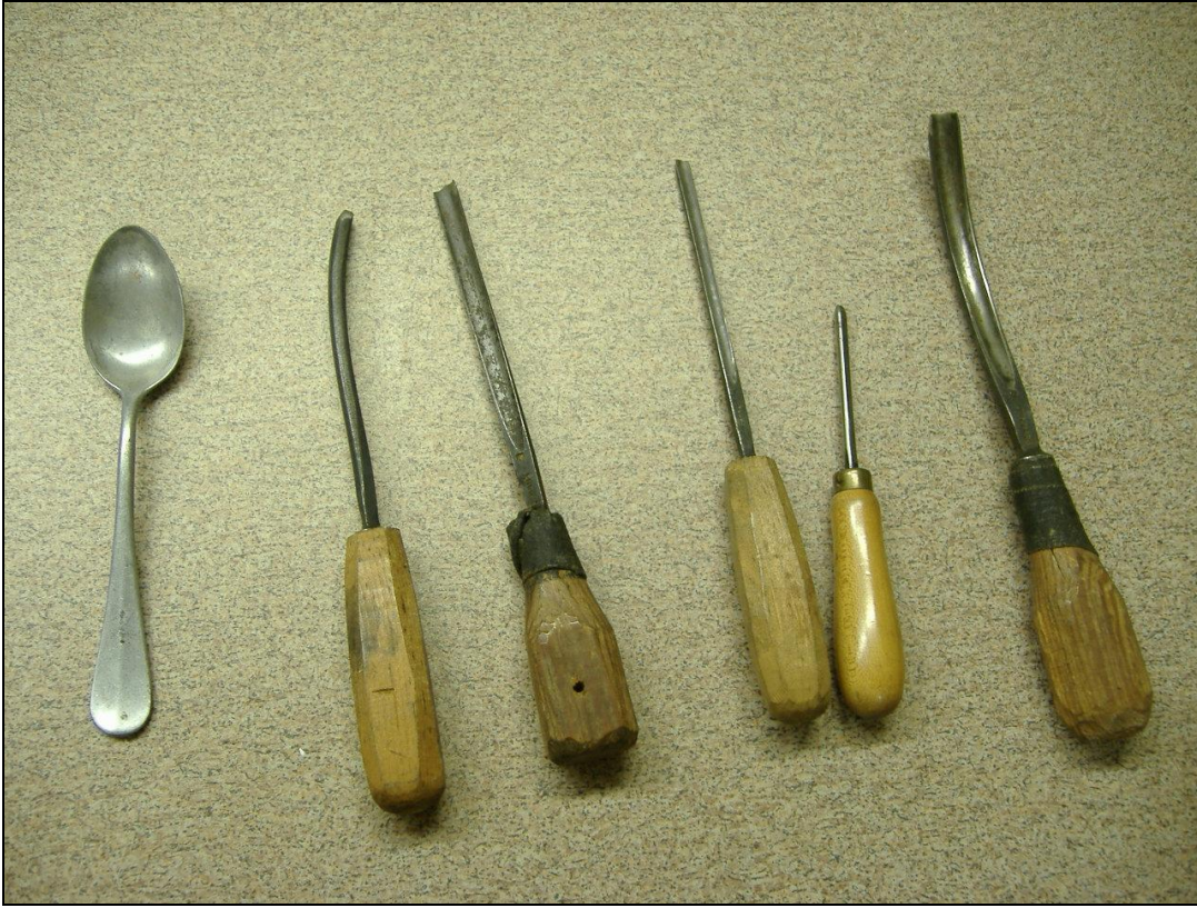
(Figure aii.2): Lazzell's wood carving tools with metal spoon used for burnishing. Photograph by Kendall Joy Martin.
