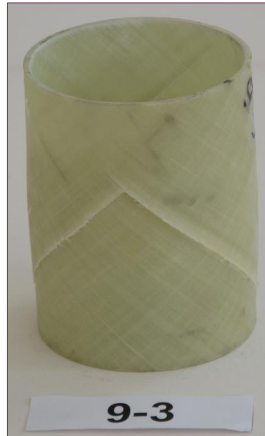
pipe specimen with 45° winding angle of the glass fibers
