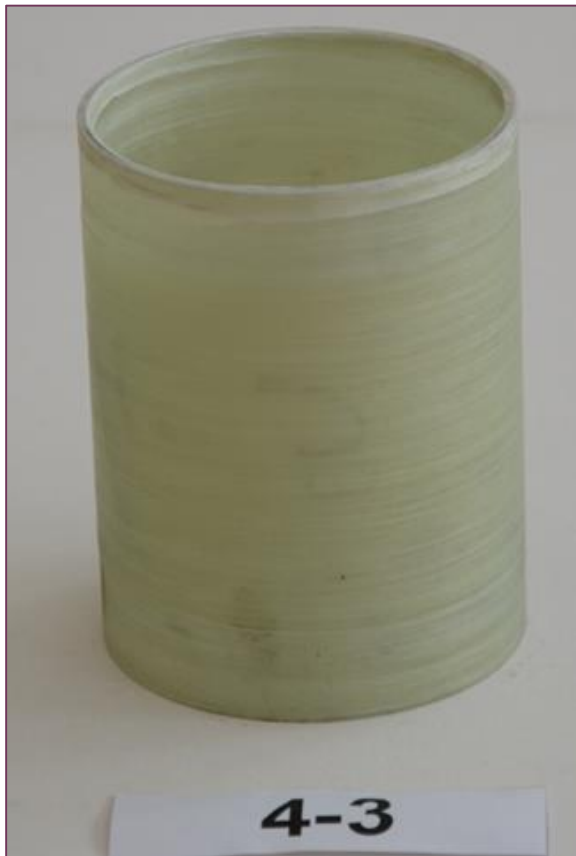
pipe specimen with 90° winding angle of the glass fibers
