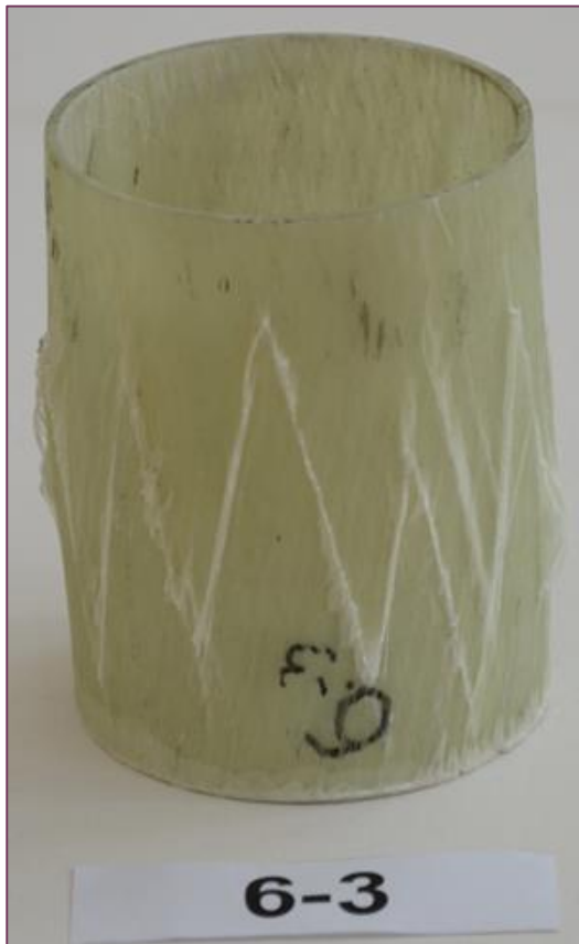
pipe specimen with 10° winding angle of the glass fibers
