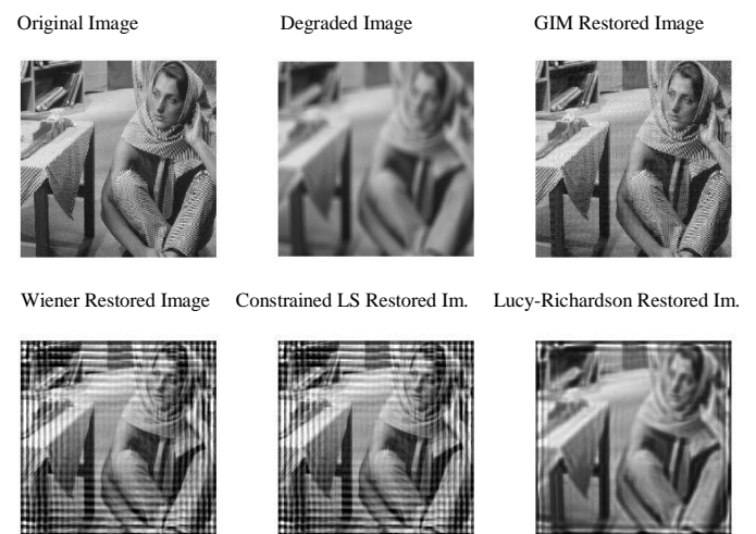
Fig. 9. Restoration in simulated degraded Barbara image for length of the blurring process l_1=15 and l_2=20 .
