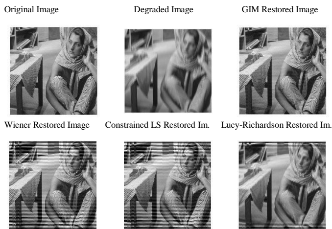
Fig. 5. Restoration in simulated vertical degraded image for length of the blurring process, l=20 .
