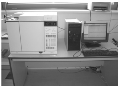
Fig. 3 Gas chromatograph Agilent GC 7890A
