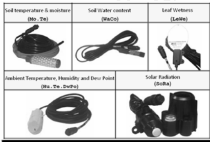
Fig. 4. The sensors of the eKo Pro wireless subsystem.
