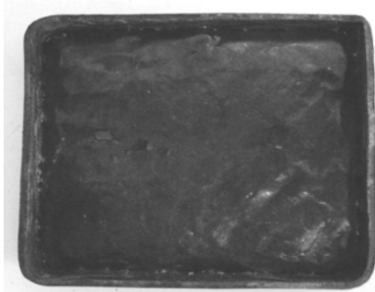
Figure 1. Green glass obtained through adding in the iron oxide elaboration batch
