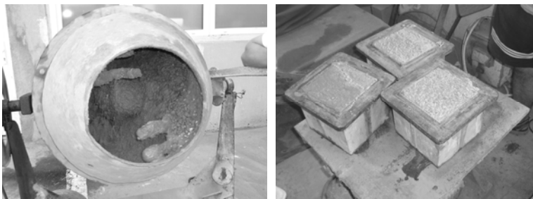
Figure. 1 Preparation of the concrete mixes.
