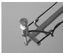
Figure 1 Microflown PU probes: PU-mini (left) placement of p and u (right) [3]
