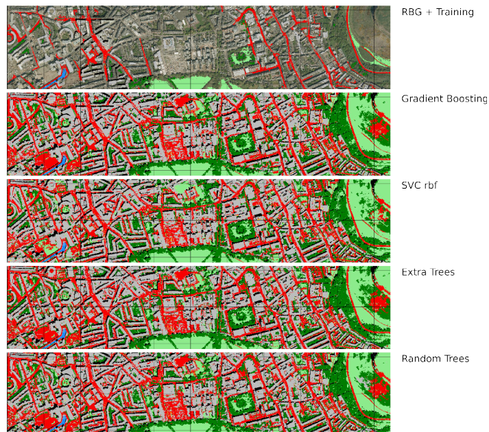
Figure 4.8: In the first plot the segments used for training the machine-learning algorithms are reported, in the other subplots the results of the classification with different algorithms are reported.
