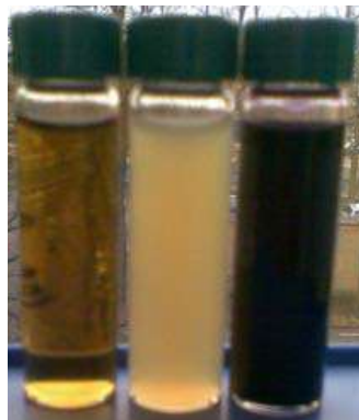
Figure 6 - Picture of a three different stabilized water based solution containing 10.0 wt. % of cerium oxide nanoparticles
