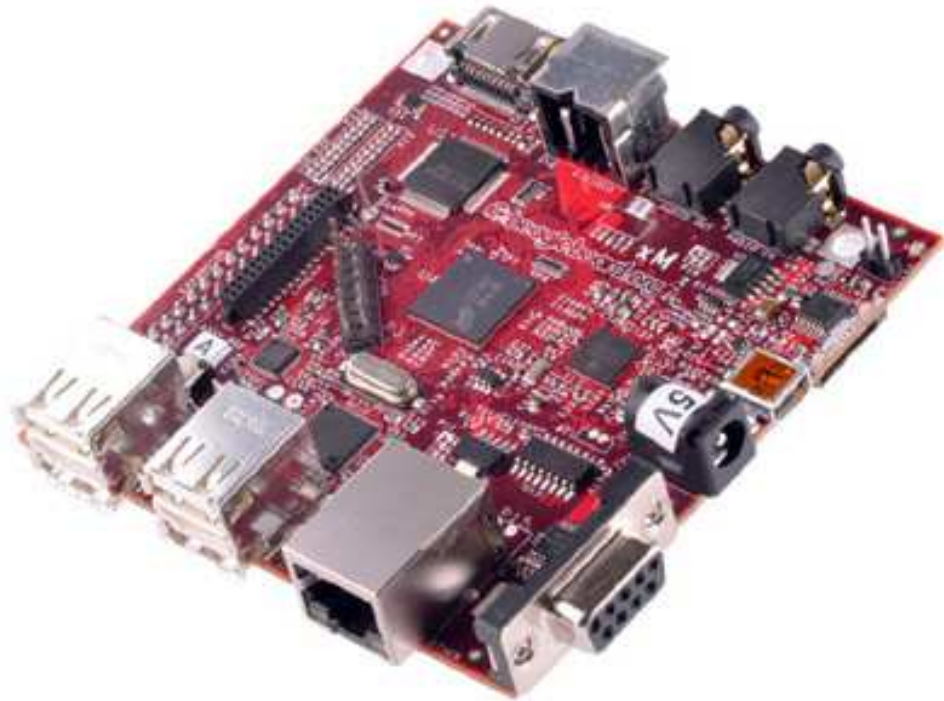
Figure 6.4: Beagleboard XM single board computer. Courtesy of http://beagleboard.org
