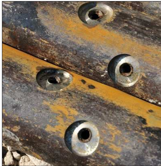
Figure 82. Exit holes in a carrier that properly resisted to the shaped charge explosions (source www.justbeneaththesurfacewv.com ).
