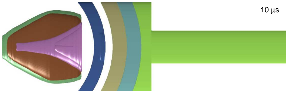
Figure 108. Eulerian FEM simulation at 10 \mu s. The needle-shaped liner is already created.
