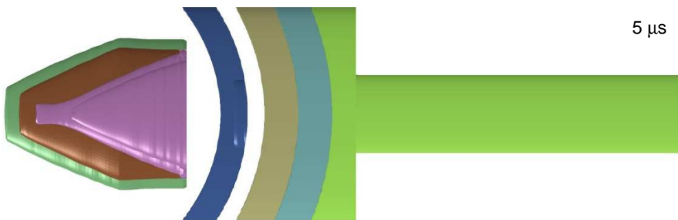
Figure 107. Eulerian FEM simulation at 5 \mu\text{s} . The shaped charge begins to expand due to the pressure from the detonation products.
