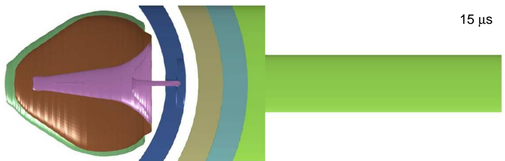
Figure 109. Eulerian FEM simulation at 15 \mu s. The liner has pierced the carrier.
