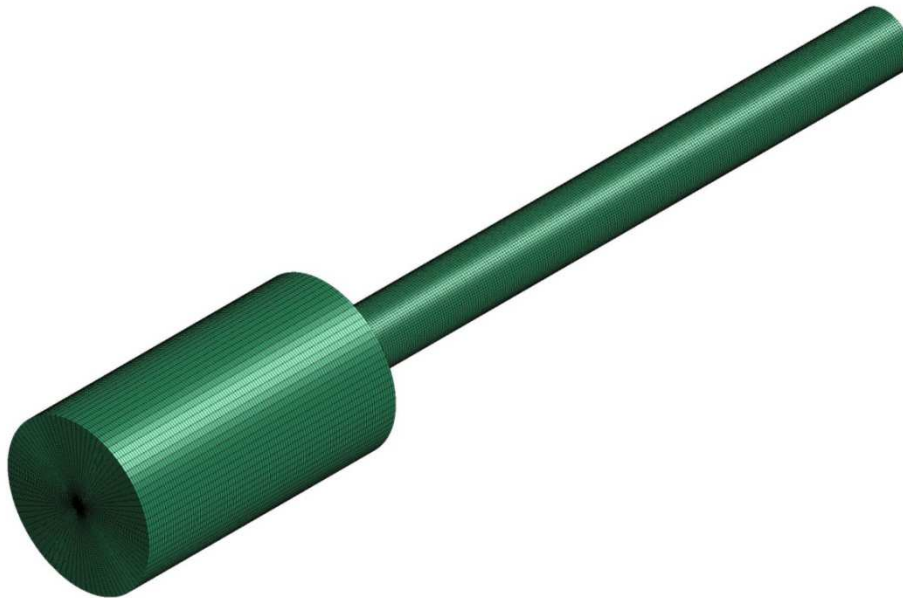
Figure 102. Single scallop Eulerian space composed of multi-material finite elements.
