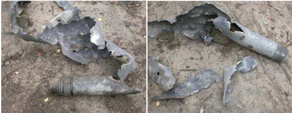
Figure 81. Total destruction of the carrier of a fired perforating gun (pictures provided by the industrial partner).
