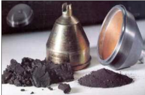
Figure 75. Components of a shaped charge (source www.slb.com ).
