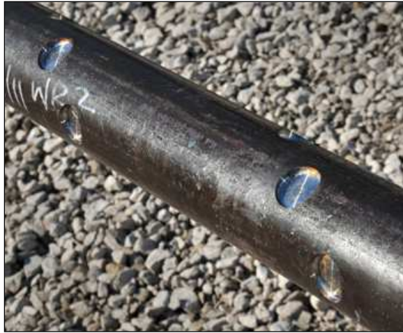
Figure 78. Scallops in an unfired carrier (source www.justbeneaththesurfacewv.com ).
