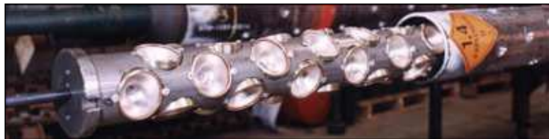
Figure 77. Insertion of shaped charges and their support and detonation systems in a carrier (source expgroup.com).
