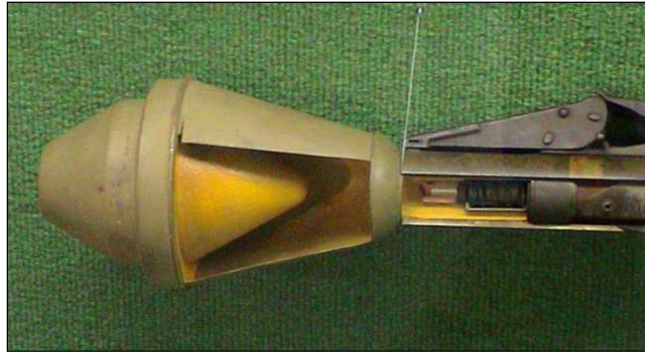
Figure 76. Shaped charge in a World War II German anti-tank weapon. The component on the left of the shaped charge is an aerodynamic cover (source defense-update.com).
