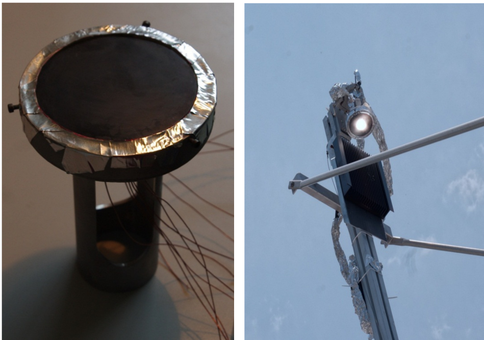
Figure A5: completely assembled flat plate calorimeter. On the right, it is mounted on the concentrator
