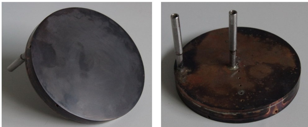
Figure A3: copper plate built as a receiver for the calorimeter: the front face has been oxidized; on the rear face, the holes for the thermocouples and inlet and outlet pipes are visible.
