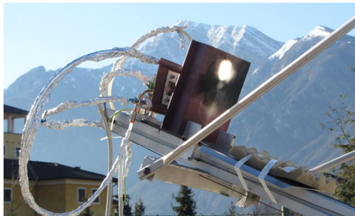
Figure 6.9: photograph of the PV receiver mounted in the focus of the concentrator. The illumination spot is focused on a protection copper shield.
