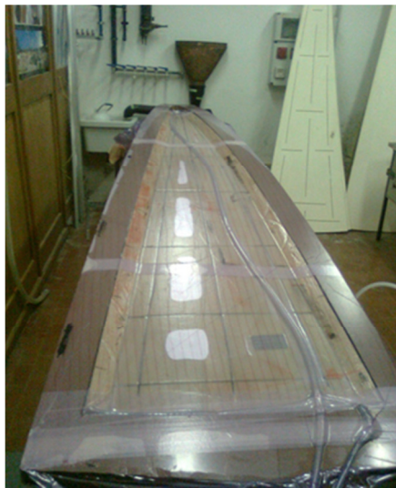
Figure 2.9: the parabolic sector placed in the mould and inserted in the plastic bag.
