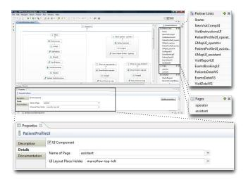
Figure 11: The extended Eclipse BPEL editor for developing UI orchestrations at work.
