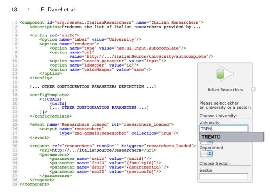
Figure. 7. The descriptor of the Italian Researchers component along with its representation in the Composition Editor
