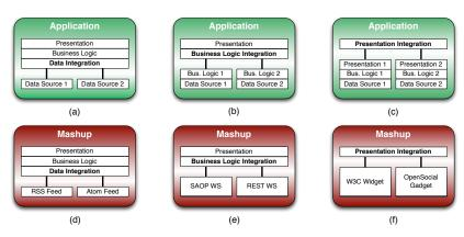
Fig. 2 The different levels of integration in general and in the specific context of web mashups.
