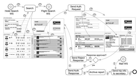
Fig. 1 Trip authorization distributed application. The gray arrows indicate synchronization or orchestration points; the number labels indicate their order in time.
