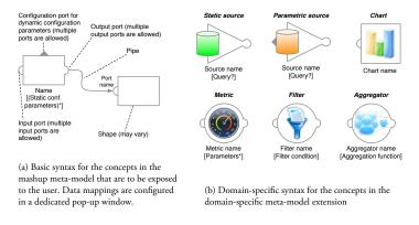
Fig. 1. Generic and domain-specific syntax for research evaluation
