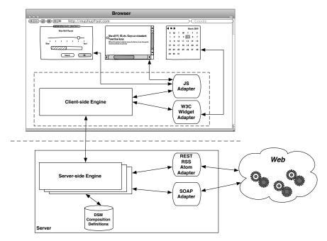
Fig. 4. Runtime environment overall architecture
