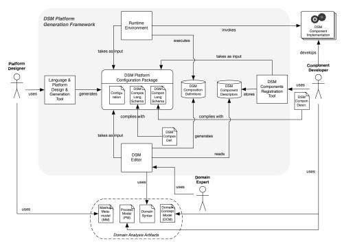
Fig. 2. Functional system architecture.
