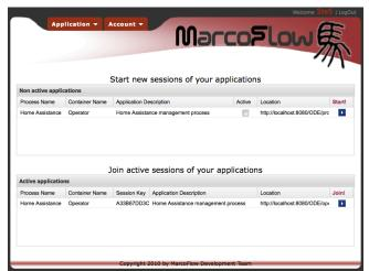
Figure 12: The management console for developers and users allowing them to deploy, instantiate, and participate in UI orchestrations.
