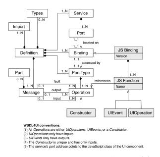
Figure 4: Simplified WSDL4UI meta-model (inspired by [23] and extended – via the gray boxes – toward UI components).
