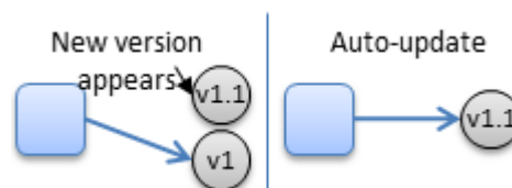
Figure 42: Auto-update example: as soon as a new version of the component appears, the system changes the "part of" annotation to point to it.
