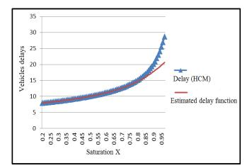
Figure 1. Delay function of the vehicles for g = 20, C = 45 and average saturation degree 0.5
