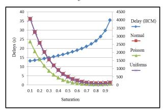
Figure 5. Delay estimates under different input distribution C = 93 and g = 45 s and average saturation X = 0.9
