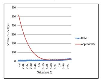
Figure 2. Delay function of the vehicles for g = 20, C = 45 and average saturation degree 0.85
