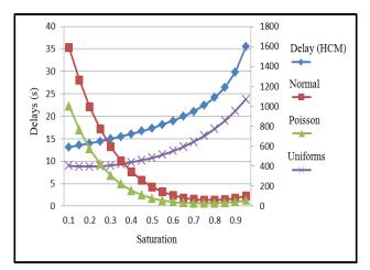
Figure 4. Delay estimates under different input distribution C = 93 and g = 45 s and average saturation X=0.85
