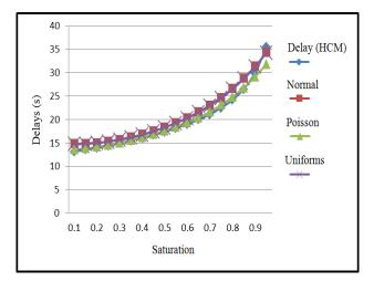
Figure 3. Delay estimates under different input distribution C = 93 and g = 45 s and average saturation X=0.5
