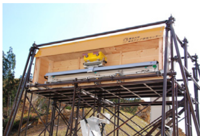
Fig. 2.11 GB-SAR system installed at the Arato-zawa site
