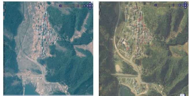
Fig. 4.2 Building Damage in Hongo after the 2011 Tsunami (left) and Pre-tsunami (right) 2
