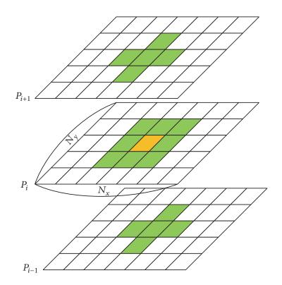
FIGURE 4.12: The data access required for the orange cell during the streaming and collision phases where Nx is the number of cells in the *x* dimension, Ny is the number of cells in the *y* direction and  $P_i$  is the *i*th plane of cells,  $0 \le i \le Nz$  where Nzis the number of cells in the *z* direction [42].
