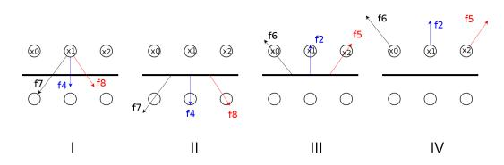
FIGURE 4.5: The procedure of the free-slip condition for the distribution functions. Notice that because the distribution functions get reflected between steps two and three, the tangential velocity along the wall is non-zero. Similar to the no-slip procedure, steps two and three are only included to give a better conceptual understanding [10].
