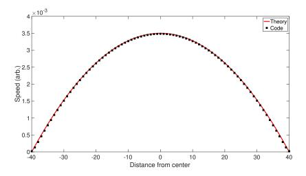
FIGURE 5.3: Comparison of the theoretical results for the Poiseuille flow from Eq. 5.4 and the results from the D3Q19 code. Notice that the simulated results agree well with the theory curve.
