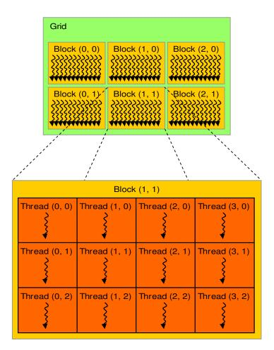
FIGURE 4.8: The breakdown of the programming model where the grid is comprised of thread blocks which are further comprised of threads. Notice that this hierarchy is similar to the architecture of the GPU itself [39].
