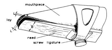
FIGURE 2.2: The clarinet reed mouthpiece system where the ligature holds the reed to the mouthpiece [14].
