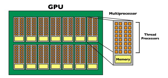
FIGURE 4.7: A graphical representation of the breakdown of the GPU into multiprocessors and thread processors. Notice that the thread processors are grouped into multiprocessors along with a limited amount of shared memory. This breakdown of the GPU computational units is analagous to the breakdown of the programming model into threads and blocks [38].
