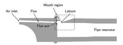
FIGURE 2.6: A diagram of the parts of a flue pipe where L is the distance from the flue exit to the labium and H is the height of the flue exit. The flue pipes studied for this thesis are closed flue pipes, so the end of the pipe resonator is closed (not pictured) [4].
