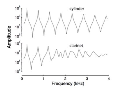
FIGURE 2.7: The impedance spectra of a closed-open cylinder and a clarinet. It can be seen that the frequency at which the peaks occur are similar for the first few peaks [18].
