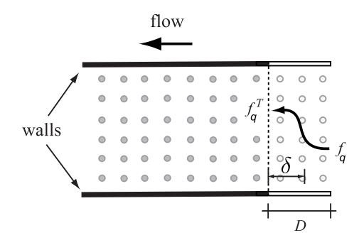
FIGURE 4.6: A schematic displaying the asymtotic target flow for the absorbing boundary condition (ABC) where *D* is the length of the buffer,  $\delta$  is the distance from the end of the buffer and  $f_q^T$  is the target distribution function. Notice that in this schematic, the target distribution function is used to asymptotically induce a source flow at the inlet of the simulation. Not pictured, it could similarly be used to set an outlet flow at the edge of the domain [9].
