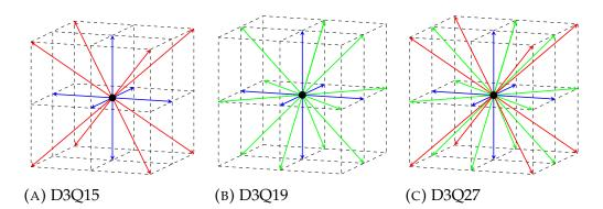
FIGURE 4.3: The lattice representations for three commonly used three dimensional lattice Boltzmann models. Notice that for all three models, the six faces of the cube are included (blue) however for 4.3a the verticies are included (red) unlike 4.3b where the edges are included (green). 4.3c includes all 27 propagation sites, the verticies, edges and faces [4].
