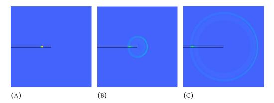
FIGURE 5.6: Results from the D2Q9 code for a pipe with an initial perturbation. Notice that the flow at the three different snapshots are similar to that of 5.5.
