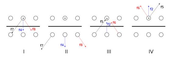
FIGURE 4.4: The procedure of the no-slip condition for the distribution functions. Notice that because the distribution function get inverted from steps two to three, the tangential velocity along the wall is zero. Steps two and three are not performed programatically, but are included as an aid to give a better understanding of the boundary condition [10].
