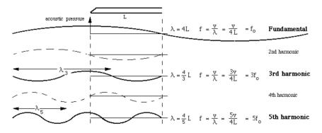
FIGURE 2.5: A representation of the acoustical pressure in a closed open tube for the first five resonance frequencies where  $\lambda$  is the wavelength, *L* is the length of the tube,  $f_0$  is the fundamental and *v* is the velocity of the wave. Notice that only the odd multiples of the fundamental are possible [18].
