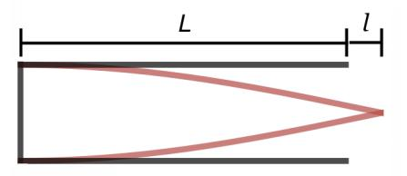
FIGURE 2.8: A representation of the pressure inside the closed open tube where the radiation impedance of the open end is nonzero with *L* being the length of the tube and *l* being the end correction.
