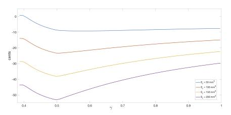
FIGURE 2.4: The results of the sensitivity analysis for the relevant surface area of the reed,  $S_r$ , where  $\gamma$  is a dimensionless blowing parameter and cents is a measure for describing ratios of frequencies. A difference of around 10 cents can be heard by the average musician, so these differing values of  $S_r$  would be audible [15].
