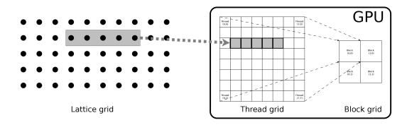
FIGURE 4.9: The mapping of the lattice grid on to the thread grid on the GPU. Notice that each lattie node corresponds with a thread on the thread grid which makes this fine-grained parallelism [10].
