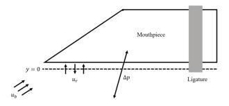
FIGURE 2.3: The clarinet reed mouthpiece system where the ligature holds the reed, dotted line, to the mouthpiece. The reed induced flow,  $u_r$ , the input flow from the muisician,  $u_b$  and the pressure difference between the inside of the mouth and mouthpiece,  $\Delta p$ , can be seen [16].
