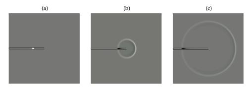
FIGURE 5.5: Snapshots of flow from a pipe with an initial perturbation from [9]. From a to b, the pulse reaches the end of the pipe where part of it reflects and part of it is radiated outwards. From b to c, the pulse continues to radiate outwards and propagate in the pipe.
