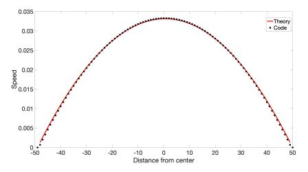
FIGURE 5.2: Comparison of the theoretical results for the Poiseuille flow from Eq. 5.7 and the results from the D2Q9 code. Notice that the simulated results agree well with the theory curve.
