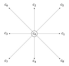
FIGURE 4.2: The lattice cell representation for the D2Q9 model where  $c_0$  is the non-propagating site and  $c_1, \ldots, c_8$  are the propagation sites. Notice that the naming convention starts with the edges of the square followed by its verticies in an anticlockwise manner.
