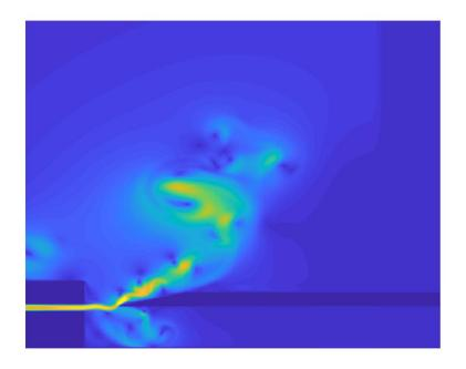
FIGURE 5.7: Flow from a flute from the D2Q9 code. Notice the presence of oscillations and vorticies about the labium.
