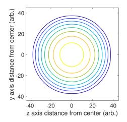
FIGURE 5.4: Equivelocity lines from the results of the D3Q19 code at an arbitrary length. Notice that the concentric circles are what is expected from Eq. 5.4.
