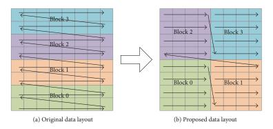
FIGURE 4.11: Two different data layout schemes: row major and tiling. While less efficient, the row major scheme is simple and still sufficiently efficient for the purposes of this thesis. For larger simulations, the increased efficiency of the tiling scheme could merit its more difficult implementation [42].
