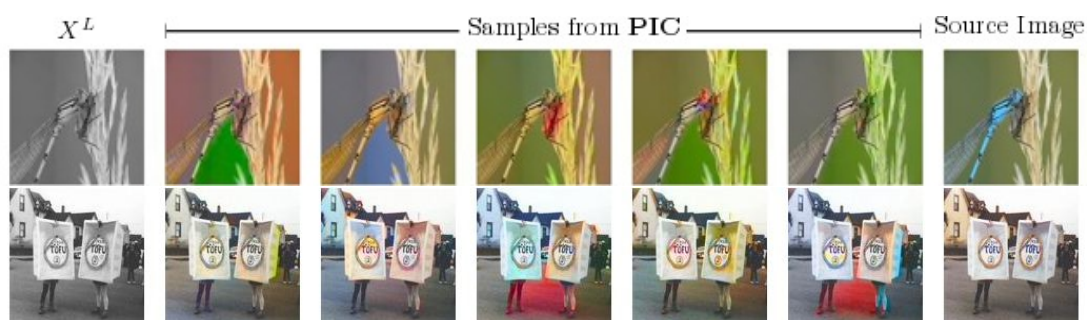
Figure 3.15: Failure cases: PIC may fail to reflect very long-range pixel interactions (top) and, e.g. , assign different colors to disconnected parts of an occluded object, or it may fail to understand semantics of complex scenes with unusual objects (bottom).
