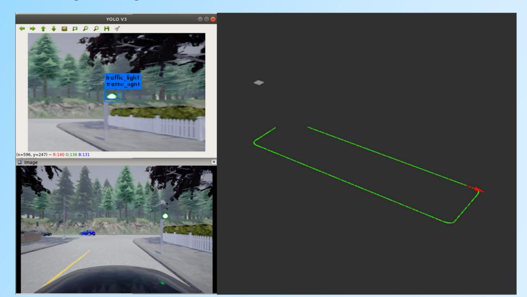
The previous picture shows YOLO image detecting a traffic light on the upper left, front image from car dashboard on the lower left and waypoints trajectory (green line) along with car position and orientation (red arrow) on the right side.
