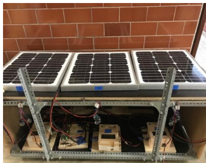
Figure 20 - Test bank using three solar panels and three controllers with different algorithms.
