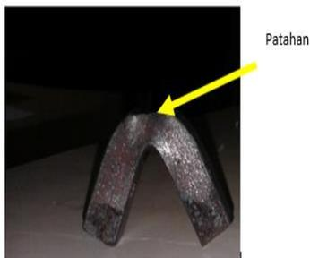
**Gambar 6 Patahan Uji Impak**
