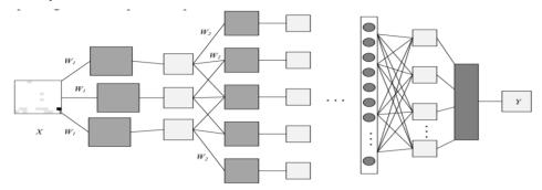
Figure 2. Convolutional neural network (CNN) structure [19]
