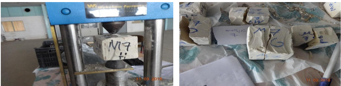
Figure 7. Samples for point load test
