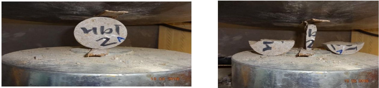
Figure 6. Samples for Brazilian (Indirect Tensile Strength) test
