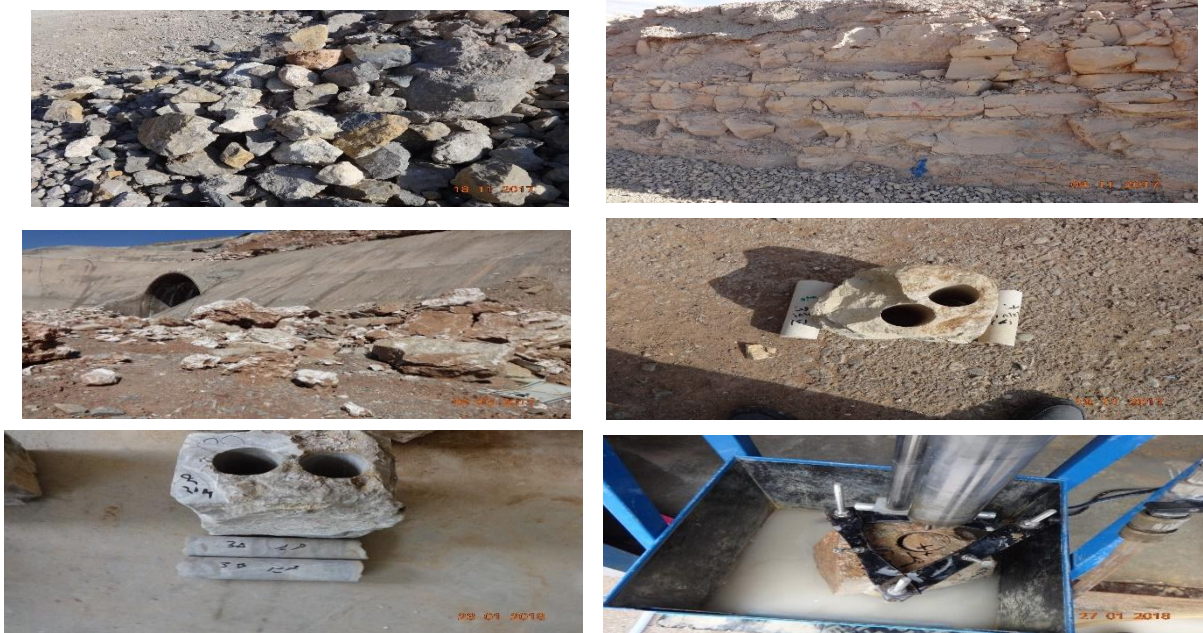
Figure 3. Sample collection and core collecting from Three tunnels locations area of study
