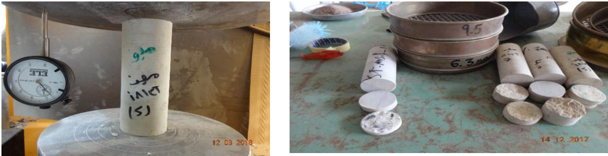
Figure 5. Samples for uniaxial compression test
