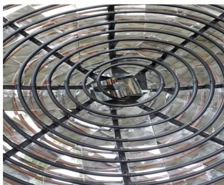
Figure 3. Shows the path of the tube, and its coating is Matte black pigment
