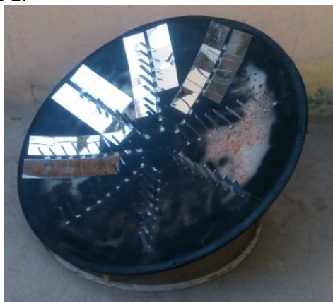
Figure 2. Shows The aluminum holders and mirrors are mounted on the concave surface
