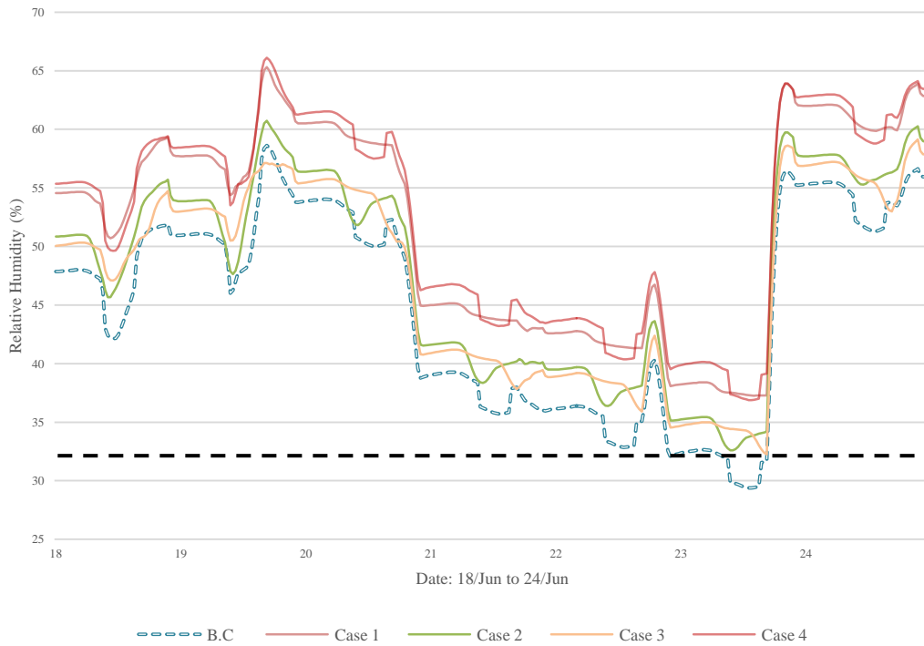
Figure 31. Relative humidity in R2 during a typical week in June for (a) zero cost ventilation strategies
