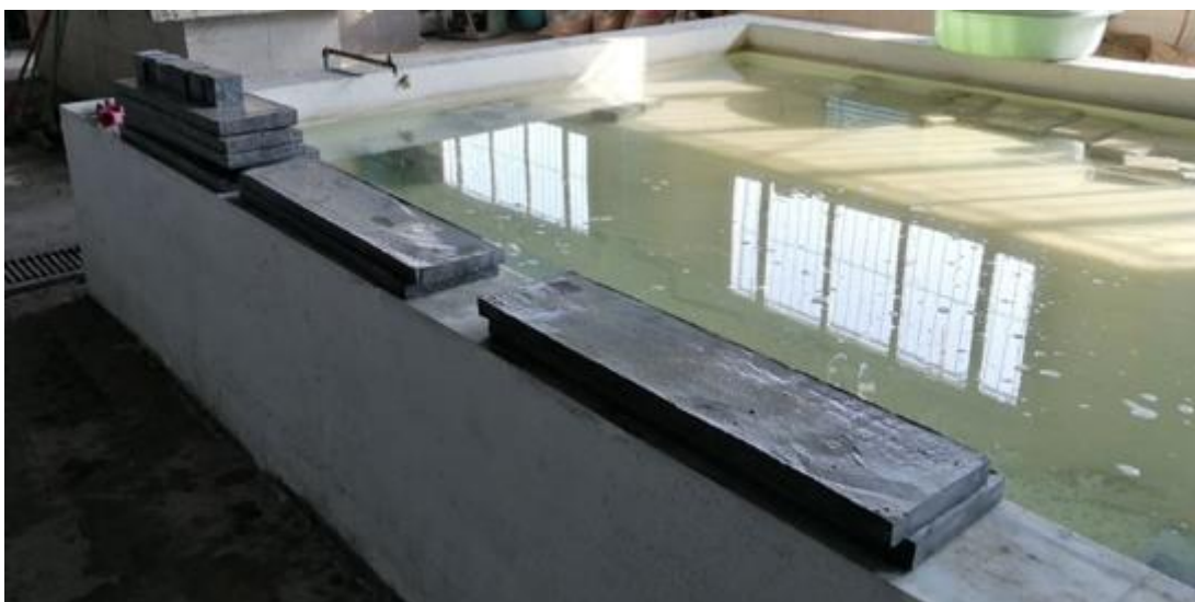
Figure 5. Drying process of ferrocement slabs after 28 days curing
