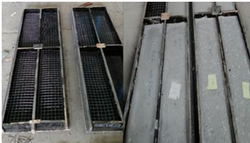
Figure 1. Reinforcing and casted fibrous ferrocement
