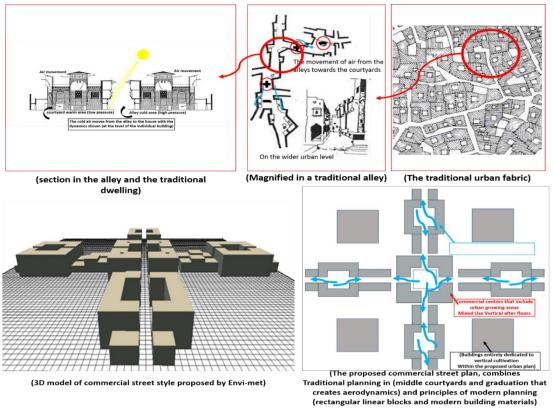
Figure 1. Low-pressure areas, the internal and external hot areas, and the Venturi action
