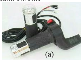
Gambar 2 (a) Hand Throttle, (b) Motor Listrik BLDC, dan (c) Baterai lithium
