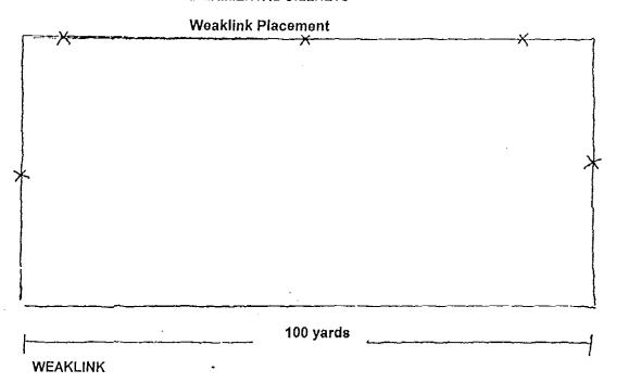
24" PIECE OF 5/16" POLY WITH OVERHAND KNOT SPLICED INTO 3/8" FLOATLINE AND TAPED OVER KNOT.
