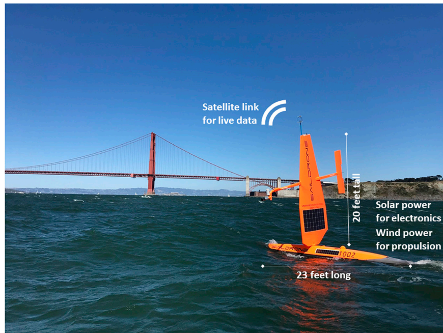
Fig. 1. The Saildrone vehicle returning to San Francisco on 11 Jun 2018. The wind anemometer is visible at the top of the wing and solar panels are on both the wing and the vehicle hull. Image credit: Saildrone/Gentemann.
