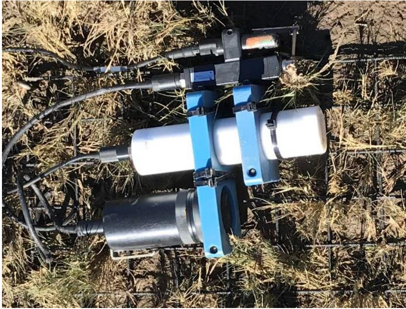
Supplementary Figure 1: An example photo of an RBR sensor deployed on the marsh surface
