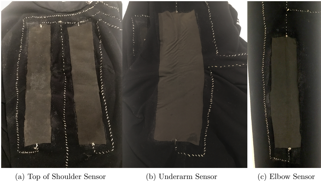
Figure 5.3: Sensor Placement Inside of Sensing Shirt
