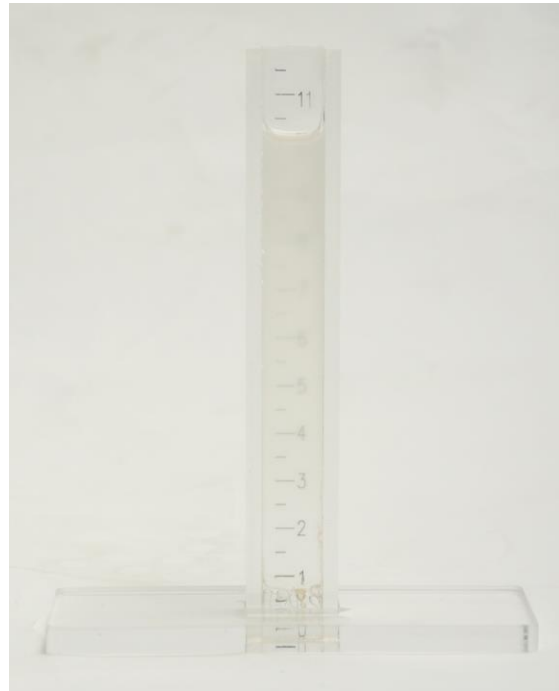
Figure 5 - Equine spermdensimeter with solution turbidity visible at number 5 on the scale under artificial light.
