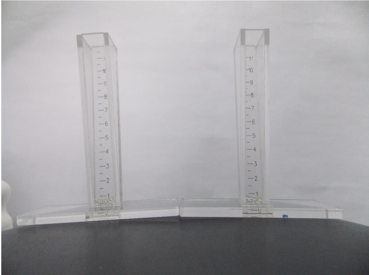
Figure 2 - Spermdensimeter prototypes developed for equine semen Models A (left, internal angle of 8°) and B (right, internal angle of 10°).
