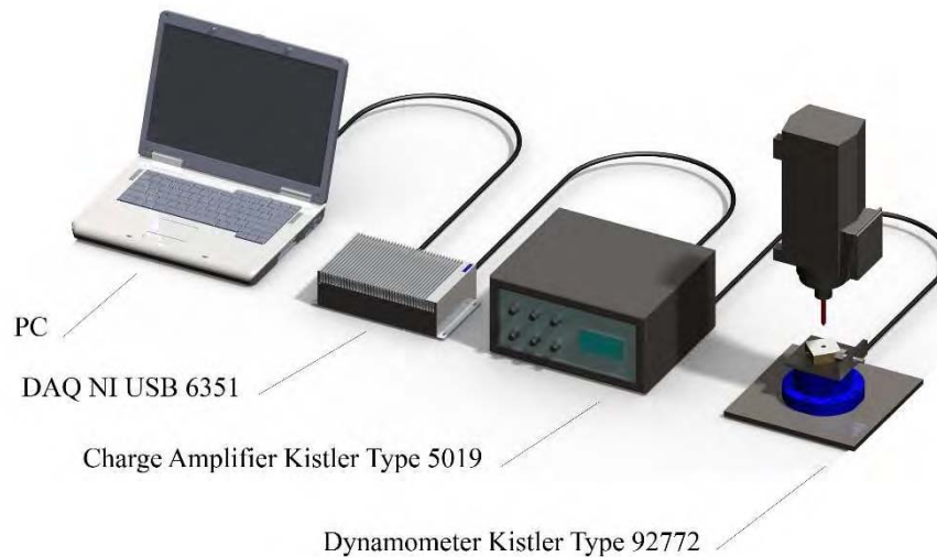
Figure 1. Measurement system block diagram
